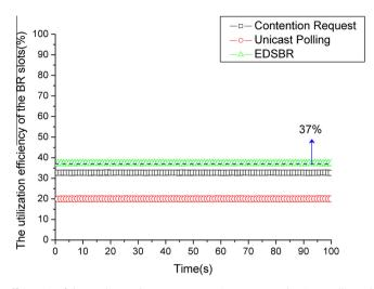
Fig. 8. Utilization efficiencies of the BR slots under EDSBR, contention request and unicast polling schemes given  $C_1 = 0.2$ .
