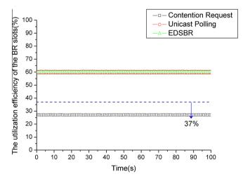
Fig. 10. Utilization efficiencies of the BR slots under EDSBR, contention request and unicast polling schemes given  $C_1 = 0.6$ .
