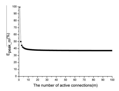
Fig. 2. Peak utilization efficiency of the BR slots in contention request mechanism given different number of active connections.
