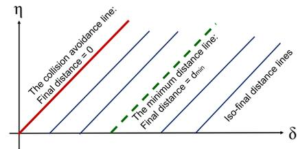
Fig. 8.  $\delta - \eta_v$  lines under a given final distance. Acceptable safety regions and collision avoidance regions can be derived from such curves.
