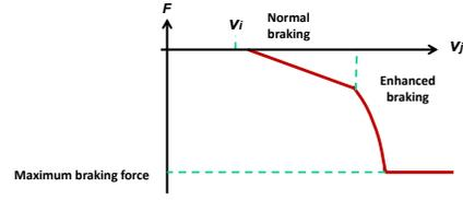
Fig. 5. Braking functions based on speed information.
