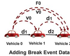
Fig. 20. Enhanced information structure by sending the braking event  $F_0$  to vehicle 2.
