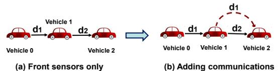
Fig. 16. Enhanced information structure by sending  $d_1$  to vehicle 2 by communication links in Example 5
