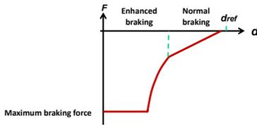
Fig. 4. Braking functions based on distance information.
