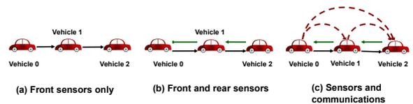
Fig. 2. Three main information structures: (a) Only front distance information is available for vehicle control. (b) Both front and rear distances are available. (c) Additional information is transmitted between vehicles.
