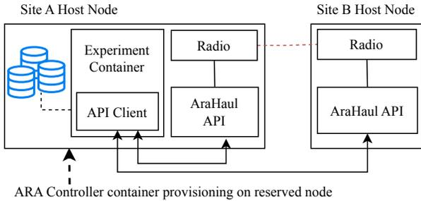
Fig. 4: Software view of the experimental setup.
