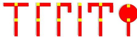
Fig. 2. The six different tools used by the robot: 1) T-stick; 2) L-stick; 3) L-hook; 4) Stick; 5) T-hook; and 6) Paddle.
