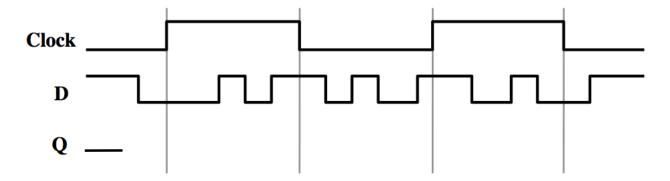
b) Complete this timing diagram a negative edge-triggered T flip-flop. (5pt)
