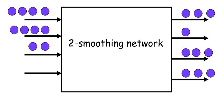
In a k-smoothing Network, the numbers of Tokens on different output wires differ by at most 2
