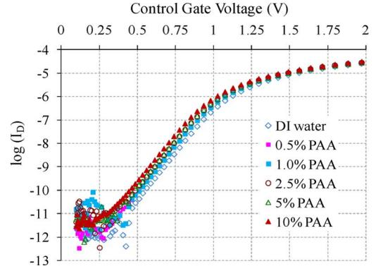
Fig. 4. Subthreshold current versus drain voltage is plotted for different PAA concentrations and compared with the DI water reference curve.
