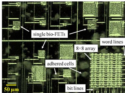
Fig. 6. Snapshot of the fabricated chip showing single and an array of biosensor devices. Cell lines placed on the chip adhered to the surface and are growing into neurons (translucent globules).
