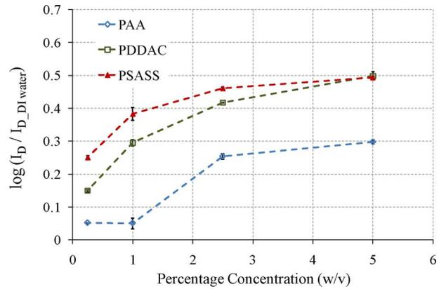
Fig. 5. Relative shift in the logarithmic drain current (difference in a device's drain current with poly amino acid and with DI water) versus percentage concentration of four poly amino acids (PAA, PDDAC, PSASS).
