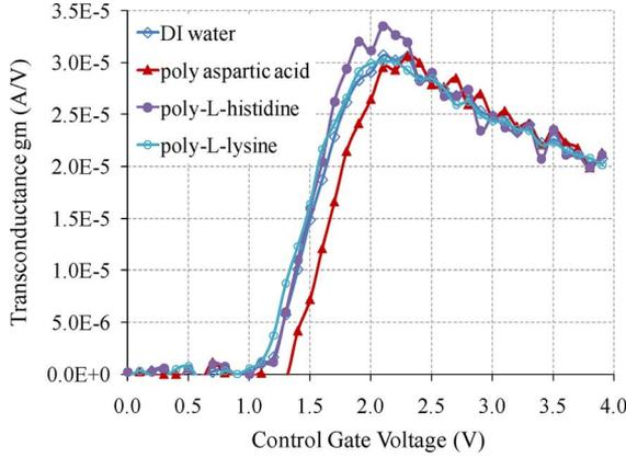
Fig. 3. Transconductance versus control-gate voltage are plotted for poly amino acids and compared with the DI water reference curve.
