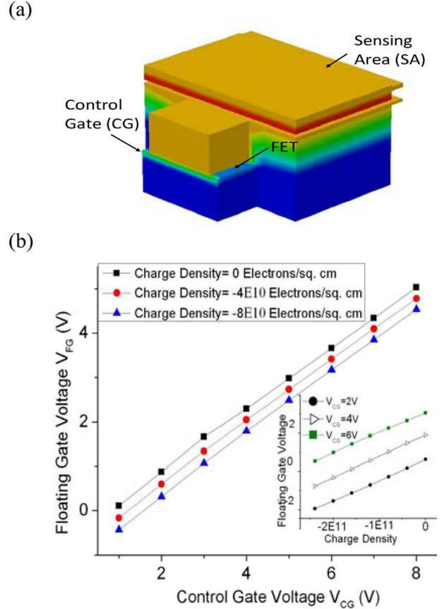
Fig. 2. (a) Three-dimensional device structure created using Sentaurus Structure Device Editor. (b) A graph of the floating-gate voltage versus the applied control-gate voltage at three fixed charge densities on the sensing area (SA). The inset shows the variation of the floating-gate voltage with charge density on the sensing area (SA) at three fixed control-gate voltages.
