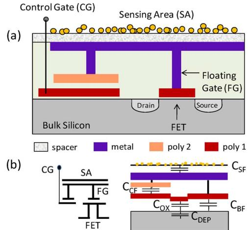
Fig. 1. (a) Structure of the proposed bio-FET showing its floating-gate, control-gate, and sensing area. (b) Equivalent capacitive model for the device.
