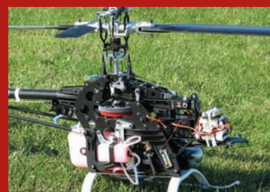
The micro UAV weighs 10 pounds and flies at speeds up to 100 mph.
