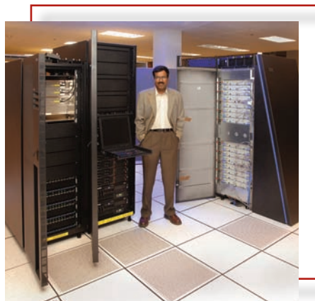
Srinivas Aluru stands next to Iowa State's CyBlue supercomputer. The IBM Blue Gene/L contains 2,048 processors and can perform 5.7 trillion calculations per second.
