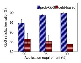
Fig. 4. QoS satisfaction ratio: prob-QoS vs debt-based algorithm with different application requirements
