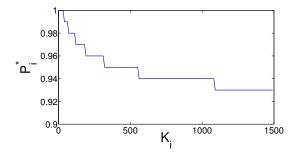
Fig. 11. An example showing the relation between  $K_i$  and  $P_i^*$ , where  $r_i$  = 0.9,  $q_i$  = 0.9999.
