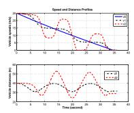
Fig. 7. Distance trajectories under slow braking.
