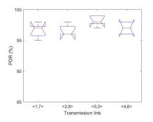
Fig. 9. Communication reliability in multi-cell scenario
