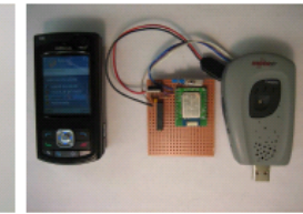
(c) A BikeNet static SAP is a WiFi AP with an Invent inserted in the USB port.
