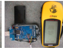
(b) An external GPS unit is attached to a Tmote Invent via its UART0 port.
