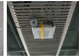
(c) A BikeNet static SAP is a WiFi AP with an Invent inserted in the USB port.
