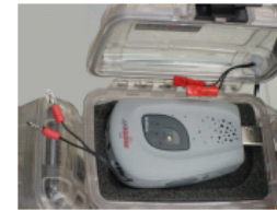
(a) A two-axis magnetometer is attached to a Tmote Invent via its ADC.
