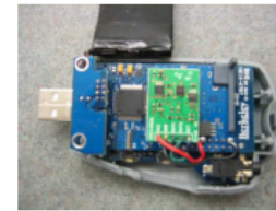
(a) A two-axis magnetometer is attached to a Tmote Invent via its ADC.
