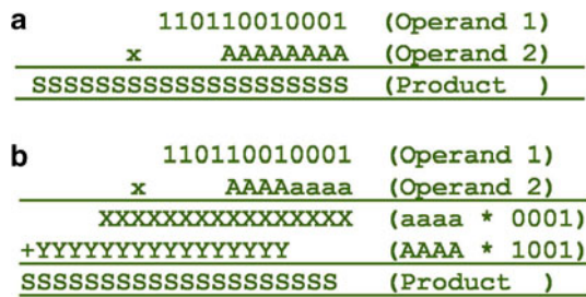
Fig. 10 Illustration of 12-bit constant multiplication with a 8-bit input. a The individual bits of product are obtained as output of a 8-LUT. b 4-LUTs are used in the implementation with the input A divided into two 4-bit values
