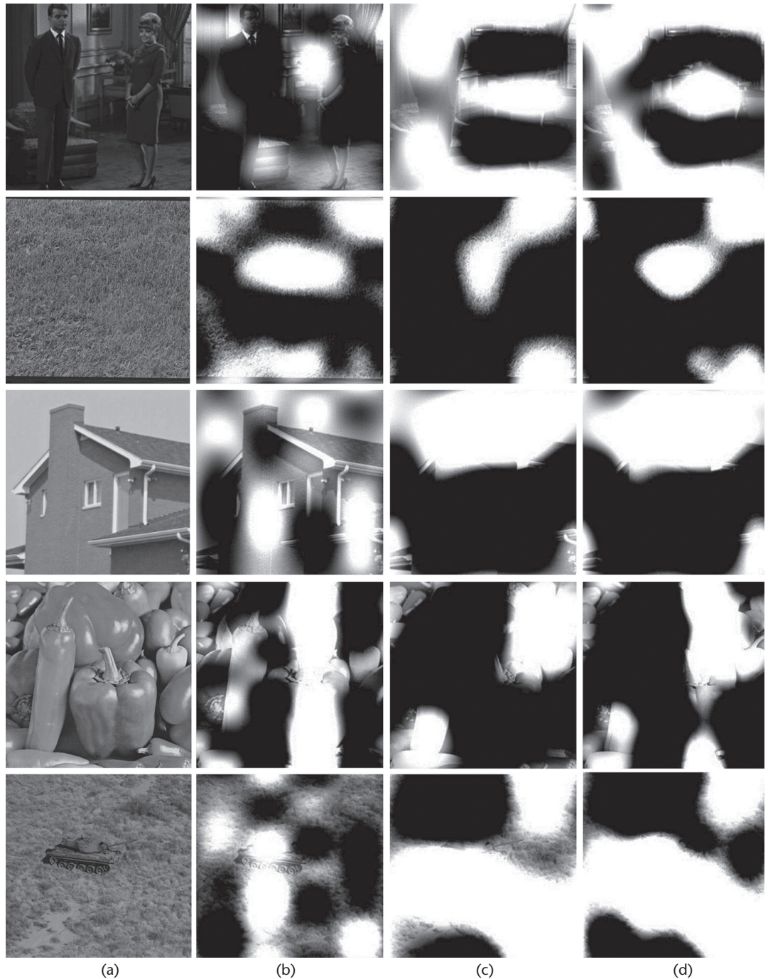
Figure 5. Image reconstruction results with selective encryption. The images were selected from the University of Southern California Signal and Image Processing Institute (SIPI) database. A selective encryption of 0.4 percent significant DWT coefficients (corresponding to sixth-level decomposition) was performed using SWT and BCAC schemes. (a) Sample images, (b) reconstruction results with SWT, (c) results with BCAC, and (d) results with SWT+BCAC.
