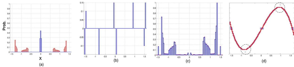
Fig. 1. (a) Invariant measure for the open-loop (in red) and the closed-loop (in blue), (b) control law, (c) Lyapunov measure  $\mu$ , and (d) structure of the open-loop (in red) and closed-loop (in blue) transitions.
