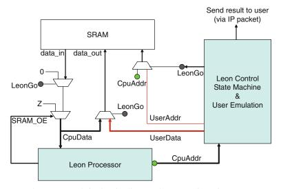
Fig. 5. External circuitry for disconnecting LEON for main memory.
