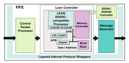
Fig. 2. High-level architecture of the Liquid processor system.
