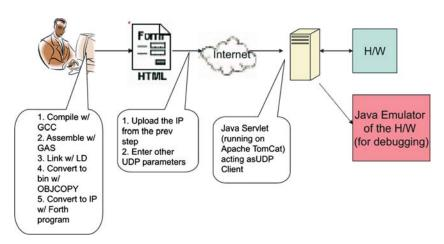
Fig. 3. Control software tool chain.
