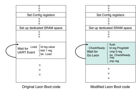
Fig. 4. Original and modified LEON Boot code.
