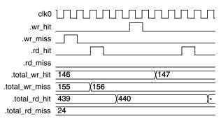
Fig. 7. Cache signals extracted from LEON.
