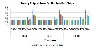
Fig. 6. This figure shows the ratio of the frequency at which the different benchmarks could have been implemented on smaller fault-free chips as compared to the maximum frequencies possible at various errors level on the larger LX110T FPGA. These tests were run for benchmarks that utilized 25% of the LX110T
