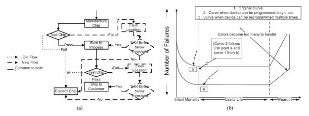
Fig. 2. (a) Changes in the manufacturing process needed to take advantage of a fault aware toolchain. These changes would increase effect chip yield according to the formula discussed in Section V-B. (b) The impact a fault aware toolchain has on the well known bathtub curve for device failure rate.
