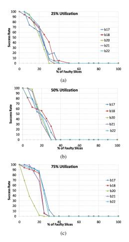
Fig. 4. The fault aware toolchain success rates for 25% - 75% device utilization. These success rates are within 1% of their actual values at a 95% level of significance.
