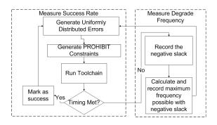
Fig. 3. The testing flow used to evaluate the proposed method.
