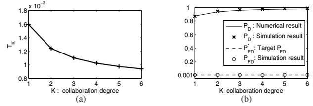
Fig. 5. (a) Normalized decision threshold ( $T_K$ ) vs. degree of collaboration ( $K$ ) when  $P_{FD}^* = 0.001$ ,  $N_K^a = 1000$ , and  $N_K^i = 3000$ . (b) Comparison of numerical and simulation results when  $P_{FD}^* = 0.001$ ,  $N_K^a = 1000$ ,  $N_K^i = 3000$ ,  $\Omega = 2100$  mW, and  $d_0 = 0.001$  units.
