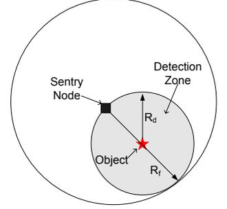
Fig. 3. Illustration of detection zone and fusion range.
