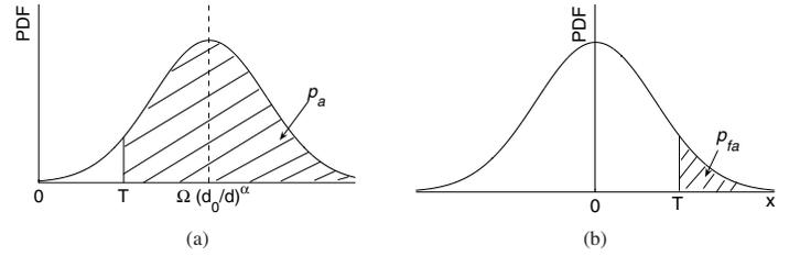
Fig. 1. (a) Probability of genuine alarm:  $p_a = P(\mathbf{x} \geq T | \mathcal{H}_1)$  and (b) probability of false alarm:  $p_{fa} = P(\mathbf{x} \geq T | \mathcal{H}_0)$ , where  $\mathbf{x}$  is the sensor measurement and  $T$  is the decision threshold.
