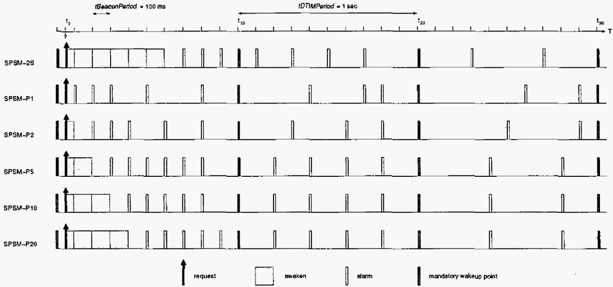
Fig. 4. Comparison of SPSM station action sequences with server RTT fixed at 10 ms
