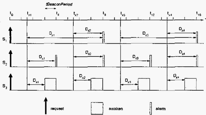
Fig. 1. Comparison of three station action sequences ( $\mathcal{S}_1$ ,  $\mathcal{S}_2$ , and  $\mathcal{S}_3$ )
