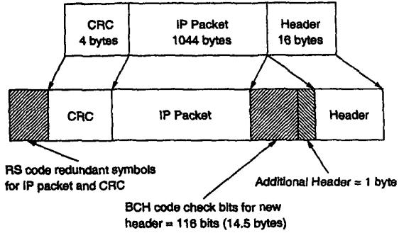
Fig. 5. Modified WaveLAN MAC frame structure
