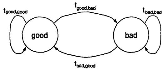
Fig. 2. Two-state Markov chain model for wireless channel
