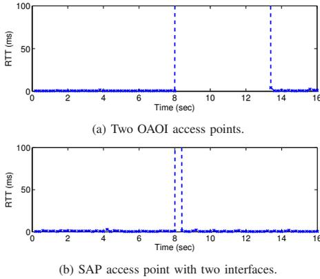
Fig. 6. Comparison of handoff delay. Handoff starts at around the 8-second mark. Large round trip time indicates packet loss.
