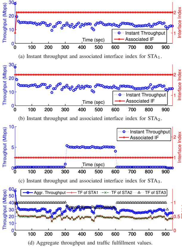
Fig. 7. Throughput and fairness performances of SAP-ST. STA<sub>1</sub> and STA<sub>2</sub> have around 30 Mbps traffic rate. STA<sub>3</sub> has time varying traffic pattern: about 200 Kbps in [0 300) sec, 6 Mbps in [300 600) sec and 200 Kbps thereafter.
