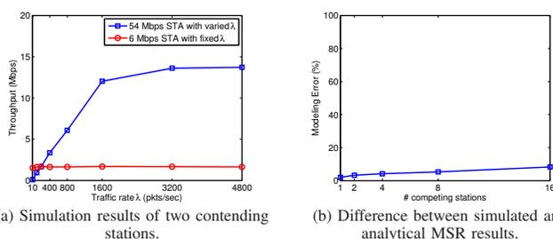
Fig. 5. Simulation-based validation of the model and algorithms for calculating the MSR.
