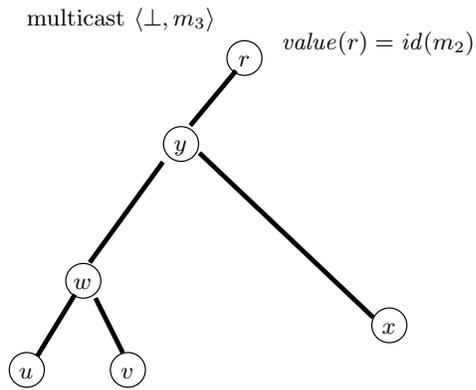
Figure 9: Combining multicast.  $m_3m_1m_2$  reaches the root.  $m_3$  is multicast as the successor of  $\perp$  (i.e.  $m_3$  is the first message in the total order). The value  $id(m_2)$  is swapped into  $value(r)$ .
