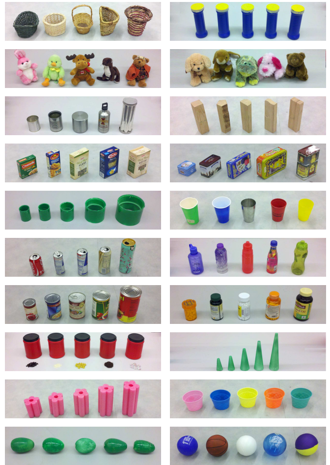
Fig. 2. The hundred objects that our robot explored. The objects are grouped according to twenty object categories. From left to right and top to bottom: 1) wicker baskets, 2) weights (objects vary by weight only), 3) small stuffed animals, 4) big stuffed animals, 5) metal objects, 6) wooden blocks, 7) pasta boxes, 8) metal tin containers, 9) PVC pipes, 10) cups, 11) pop cans, 12) plastic bottles, 13) canned food, 14) medicine pill bottles, 15) coffee containers with different types of contents, 16) green cones, 17) pink noodles, 18) egg coloring cups (vary only by color) 19) easter eggs (vary by material, and 20) balls.
