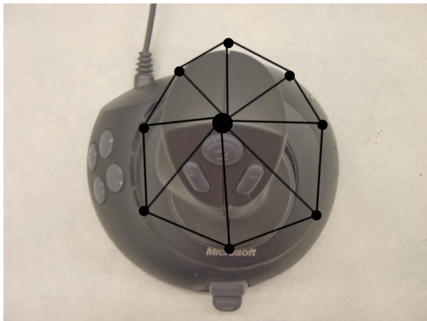
Figure 6: Points are sampled around the functional area of the joystick by selecting a random point within a triangle that is formed by taking two consecutive points along the outer polygon displayed in this image and the center point. This region is assumed to be convex in \mathbb{R}^7 .
