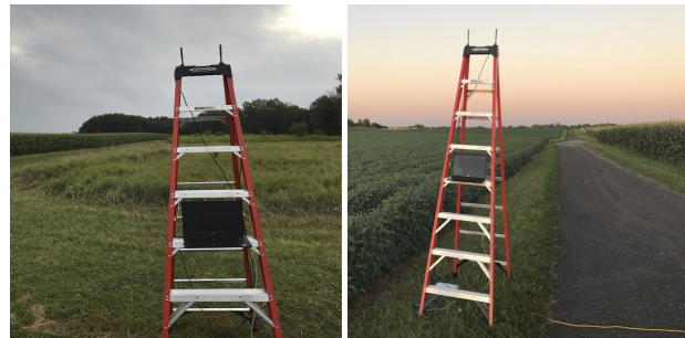
Fig. 5: MIMO antennas mounted of top of the ladder
