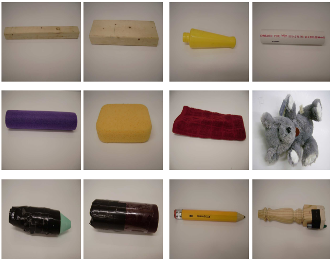
Fig. 2. The twelve objects used in the experiments and their corresponding material types: (row 1) 2x2 and 2x4 (wood); plastic toy and PVC pipe (plastic); (row 2) noodle and sponge (sponge); hand towel and teddy bear (cloth); (row 3) sidewalk chalk and wax candle (soft materials); oversized pencil, whiteboard marker attached to a piece of wood to make it graspable (common writing instruments). Shown not to scale.
