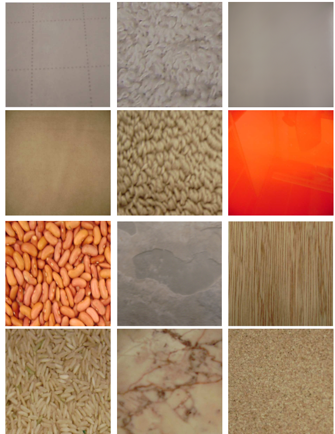
Fig. 3. The twelve surfaces used in the experiments shown in vertical pairs of two along with their material types: (column 1) wrapping paper and cardboard (paper); beans and rice (deformable surfaces formed of small objects); (column 2) towel and rug (cloth); terracotta tile and marble (stone); (column 3) whiteboard and plexiglass (plastic); wood and bulletin board (wood).
