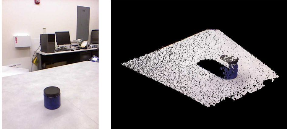
Figure 3.5 Example RGB image and its corresponding 3D point cloud captured by the robot's Microsoft Kinect sensor.
