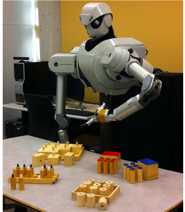
Fig. 1. The robot and the four Montessori matching tasks that were used in the experiments. In clockwise order, the four tasks were: sound cylinders, weight cylinders, pressure cylinders, and sound boxes.
